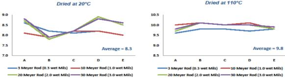
Coated Matte Acrylic onto 2A Leneta Card, with various Meyer Rods and Dried at various Temperatures
